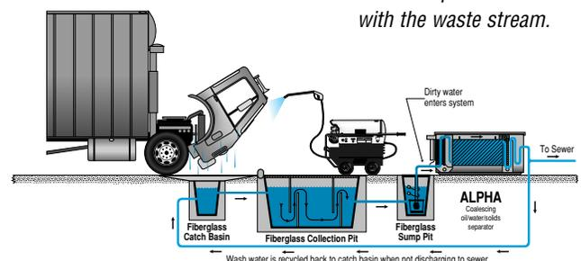
**The Alpha can work in conjunction with below-ground catch basins and collection pits or as a stand-alone oil-water separator.**
